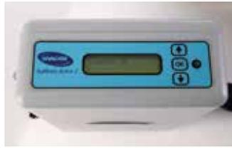
“Intelligent” software in the pump will identify and advise pump status via the LCD screen.
