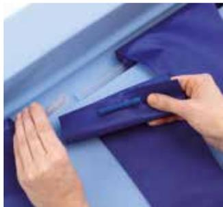
In case of accidental puncturing, individual air inserts can be easily replaced.
